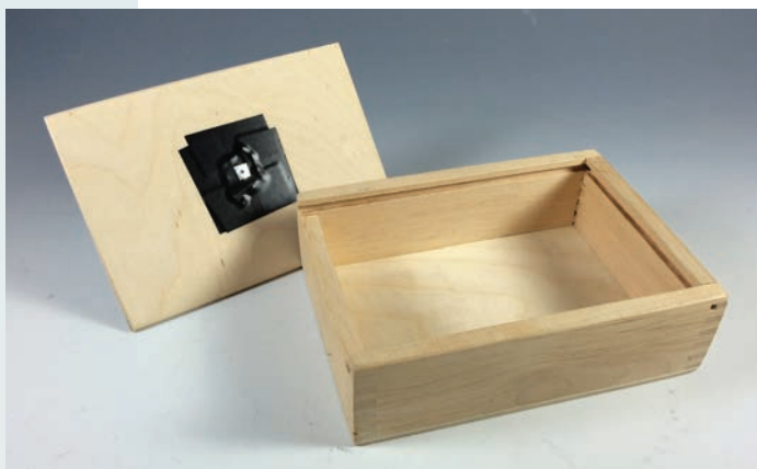
Fig. 1-46. Aluminum pinhole is taped in place over the sub-hole.
