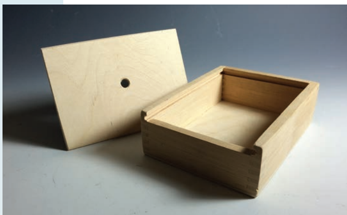
Fig. 1-45. Light-tight box before the interior is painted black.
